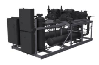
intended for facilities that require cold storage or combined freezer and cold storage. Using the combination reduces the ammonia charge by up to 90% as compared to ammonia only systems. Carbon Dioxide is non-flammable, non-toxic and has an Ozone Depletion Potential (ODP)=0, and has a Global Warming Potential (GWP)=1.
